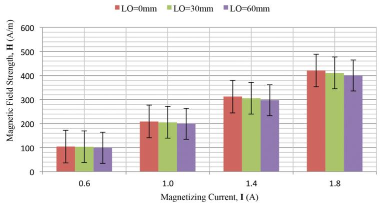
FIGURE 2. Field strength distribution for different sample's dimension, grade M4
