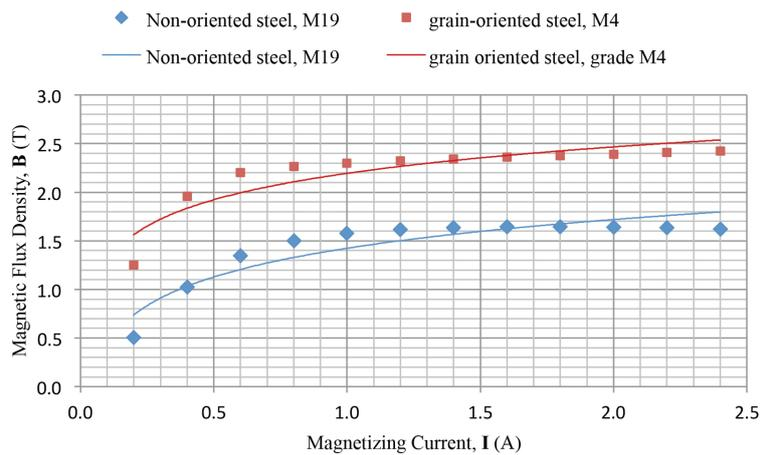
FIGURE 4. Magnetic flux density for electrical steels, grade M4 and M19
