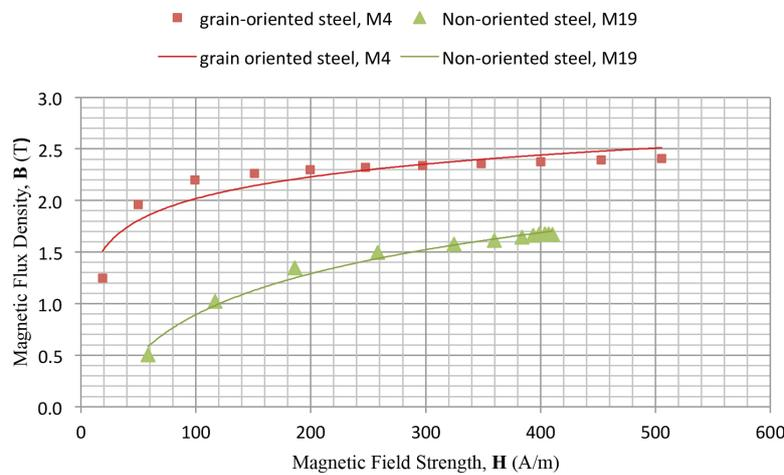
FIGURE 6. Magnetization curves of electrical steels, grade M4 and M19
