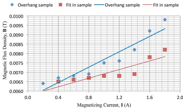
FIGURE 3. Flux distributions of normal stray flux at the center of sample, grade M4
