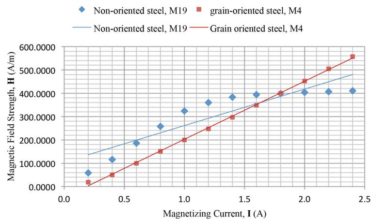
FIGURE 5. Magnetic field strength for electrical steels, grade M4 and M19
