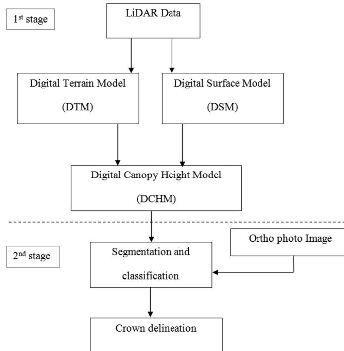
FIGURE 2. Workflow and data processes of canopy delineation from LiDAR data
