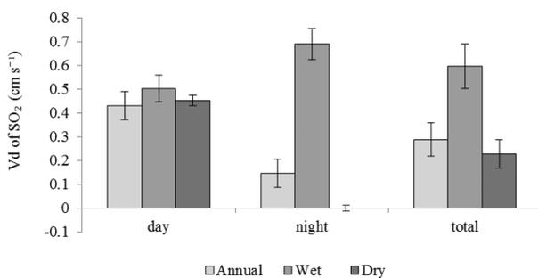
FIGURE 3. Dry deposition velocity of SO<sub>2</sub> evaluated using the aerodynamic gradient method
