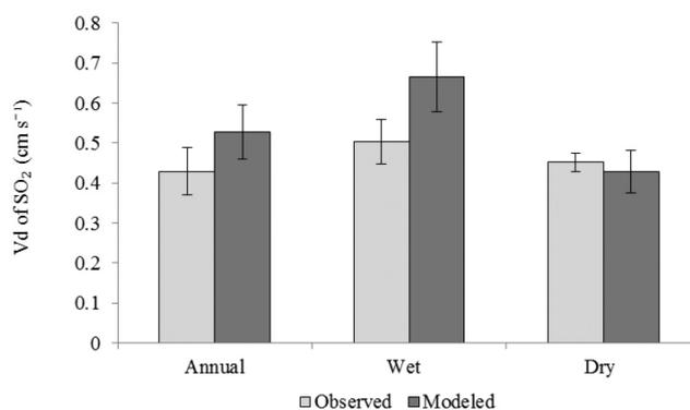
FIGURE 5. Comparison of the dry deposition velocity of SO<sub>2</sub> determined by the aerodynamic gradient method with that determined using the resistance model
