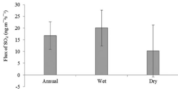
FIGURE 2. Dry deposition flux of SO<sub>2</sub> evaluated using the aerodynamic gradient method
