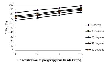
FIGURE 4. Cuttings transport ratio against weight concentration of polypropylene beads in the water-based mud
