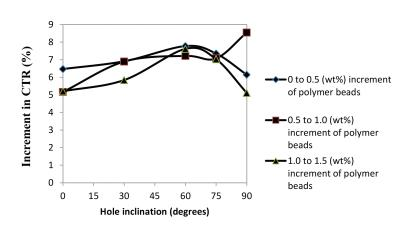
FIGURE 5. Incremental cuttings transport ratio against incremental changes in wt. % of polypropylene beads
