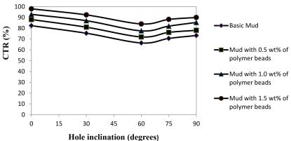
FIGURE 3. Cuttings transport performance for respective muds
