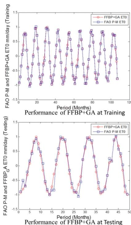
FIGURE 5. The correlation between calculated ET<sub>0</sub> using FAO P-M equation and FFBP+GA predicted ET<sub>0</sub> during training and testing stage for Baghdad station
