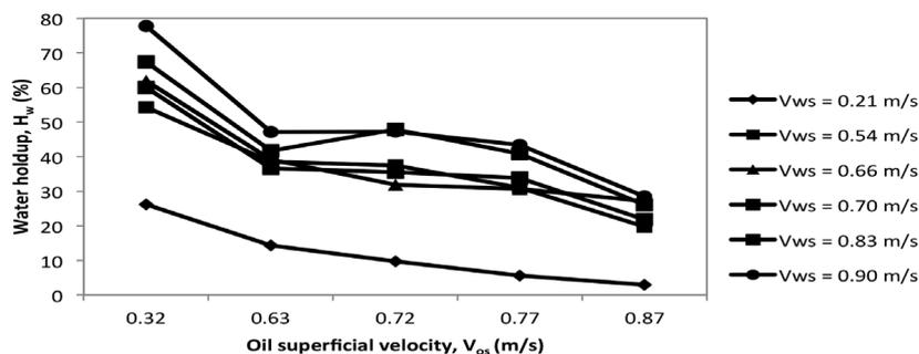
FIGURE 6. Water holdup vs. superficial velocities of oil and water
