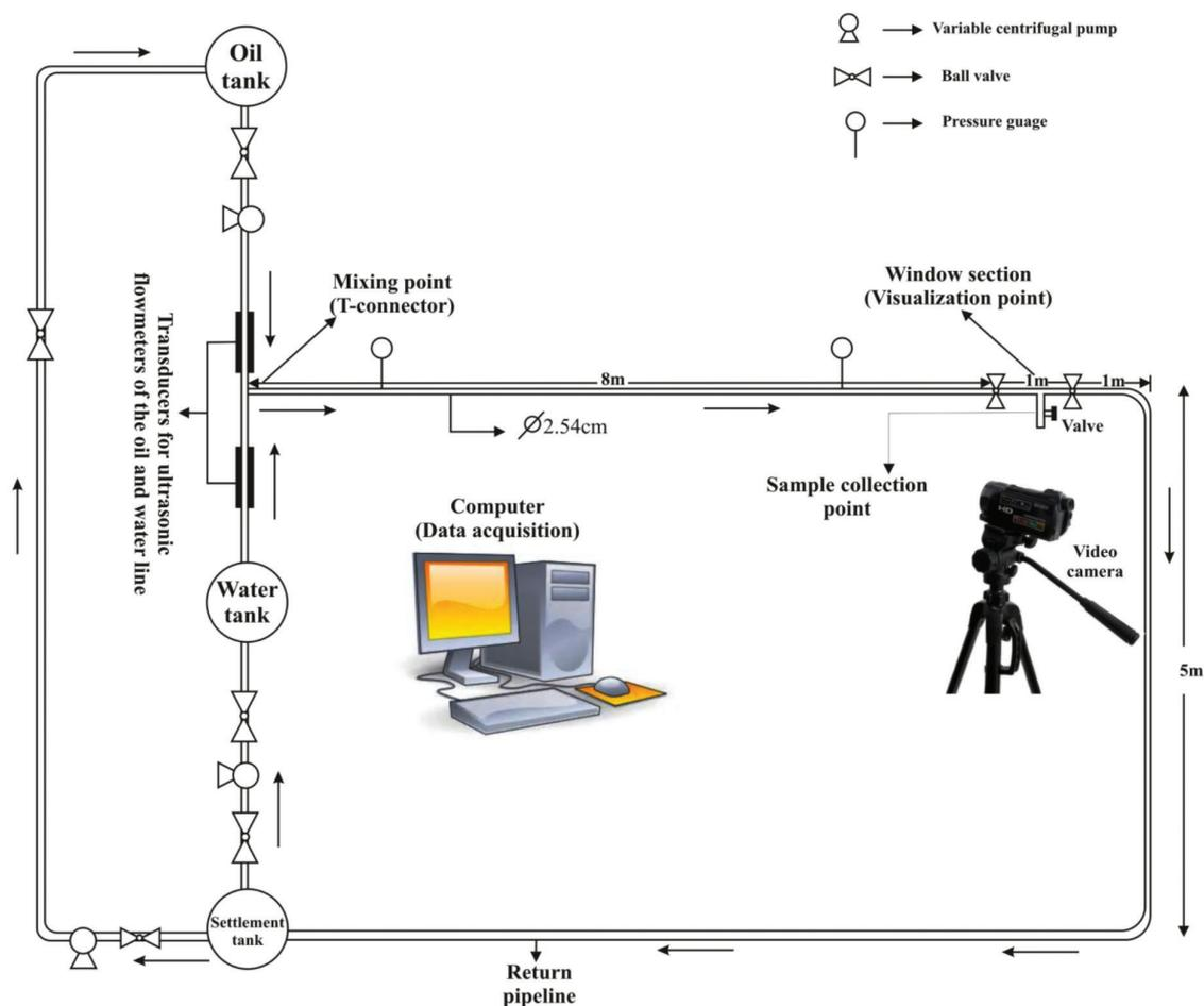
FIGURE 1. Schematic diagram of the experimental flow setup
