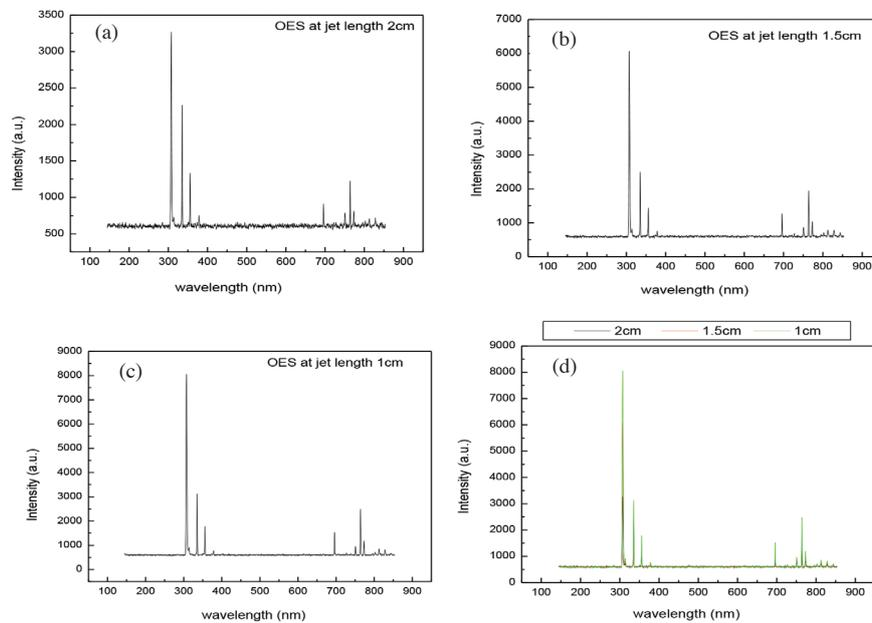
FIGURE 3. Optical emission spectra of atmospheric pressure plasma jets with different jet lengths
