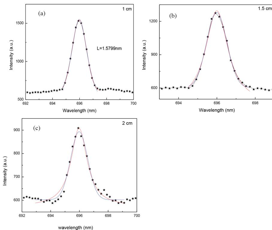
FIGURE 5. Magnified profiles of spectral lines for the determination of full width at half maxima (FWHM)
