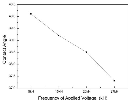
FIGURE 12. Water contact angle as function of frequency of applied voltage for fixed treatment time
