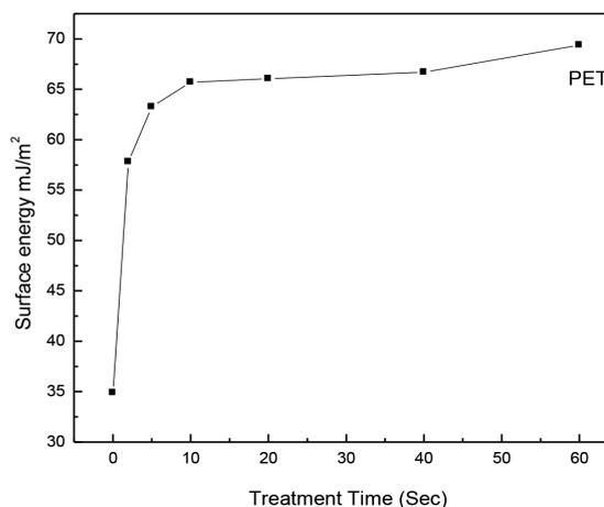
FIGURE 11. Surface energy of PET as function of treatment time. The sample was placed at 3.5 cm from the nozzle jet length 3.5 cm
