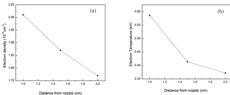
FIGURE 6. (a) Electron temperature,  $T_e$  and (b) electron density  $n_e$  as a function of distance along the jet length
