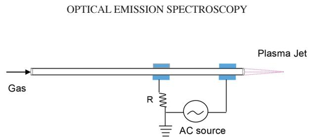
FIGURE 1. Schematic of the experimental configuration of atmospheric pressure plasma jet
