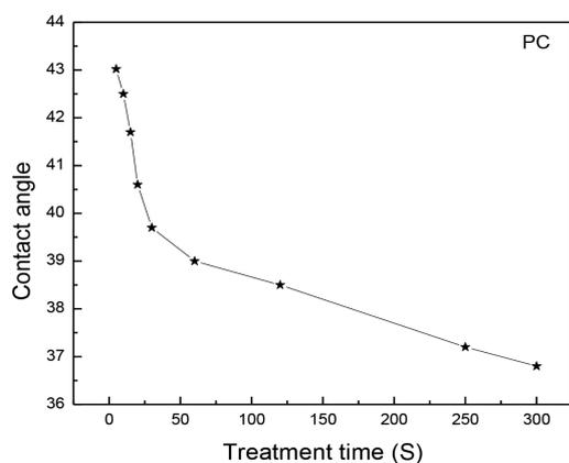
FIGURE 8. Water contact angle on PC as function of treatment time in APPJ in argon. The sample was placed 3.5 cm from the nozzle
