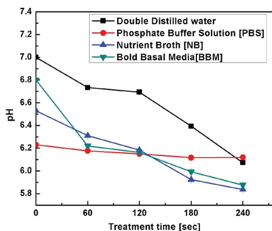
FIGURE 13. pH of different liquids as function of treatment time
