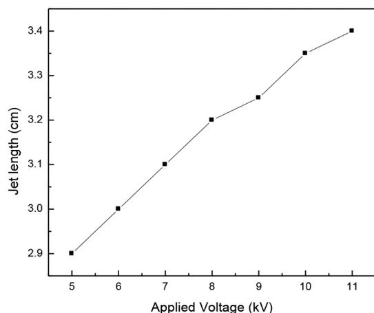
FIGURE 7. Plasma jet length as a function of applied voltage
