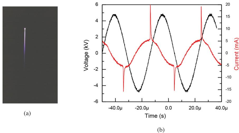
FIGURE 2. (a) a photographic image of the plasma jet and (b) electrical signals of the discharge
