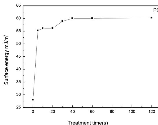
FIGURE 10. Surface energy of PC as function of treatment time. Sample was placed at 3.5 cm from nozzle
