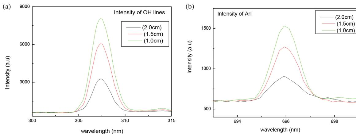
FIGURE 4. Intensity of OH and Ar-I spectral lines at different position of plasma jet
