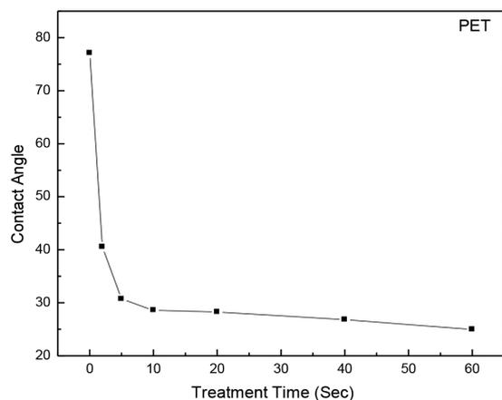
FIGURE 9. Water contact angle on PET as function of treatment time in APPJ in argon. The sample was placed 3.5 cm from the nozzle
