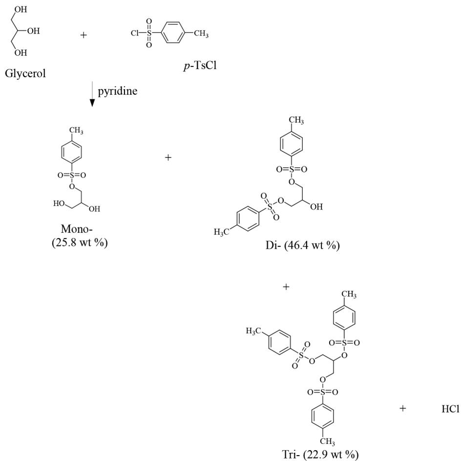
FIGURE 1. Tosylation process of glycerol with *p*-TsCl in the presence of pyridine
