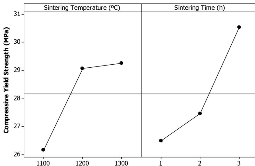
FIGURE 4. Main effect plot for the compressive yield strength of stainless steel foams
