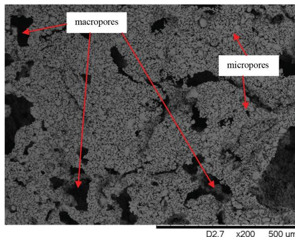
FIGURE 1. Scanning electron micrograph of stainless steels foam
