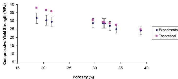
FIGURE 3. Effect of porosity on the compressive yield strength of stainless steel foams
