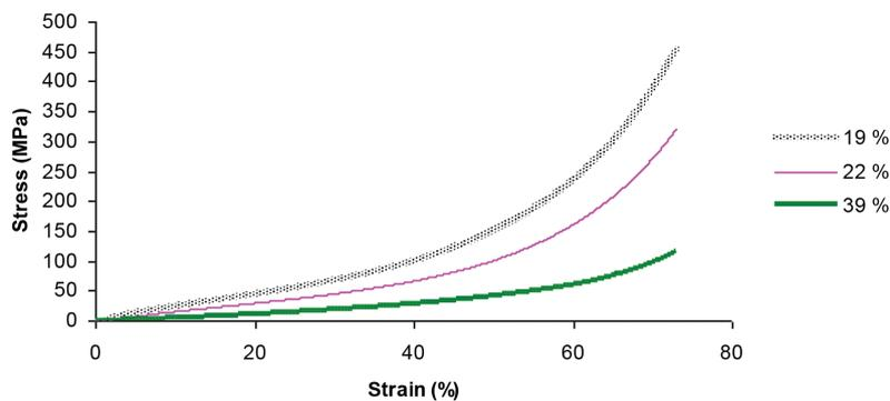
FIGURE 2. Compressive stress-strain curves for stainless steel foams with different porosities (sample with porosity 19% carried out at 2 h, 1200°C; porosity 22% carried out at 3 h, 1100°C and porosity 39% carried out at 1 h, 1100°C)
