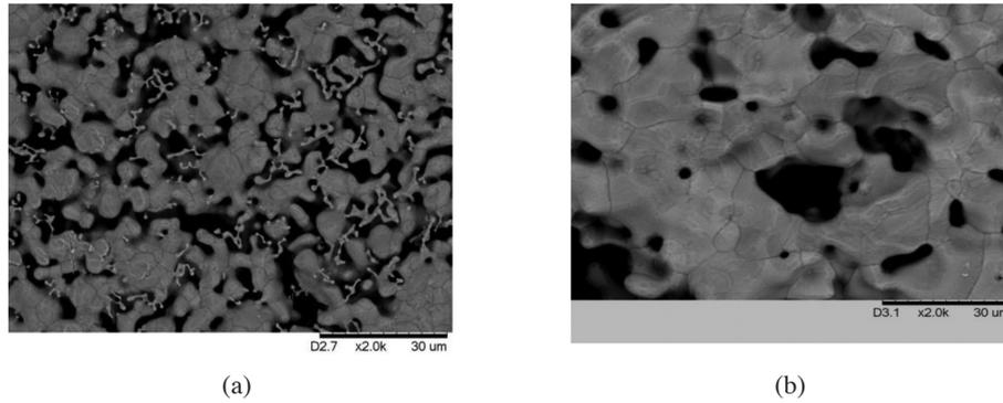
FIGURE 5. SEM images of stainless steel foams sintered at different temperature for 1 h (a) 1100°C and (b) 1300°C
