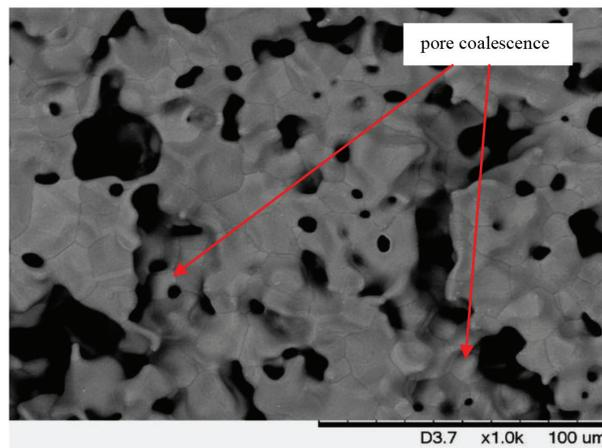
FIGURE 6. SEM image of stainless steel foam sintered at 1300°C for 3 h
