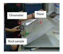
FIGURE 5. A self-fabricated tilt testing apparatus, modeled after Priest (1993) used for measurement of peak friction angle,  $\phi_{neak}$
