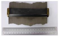
FIGURE 3. Standard 15 cm Barton comb used to reproduce the true roughness profiles of discontinuity surfaces
