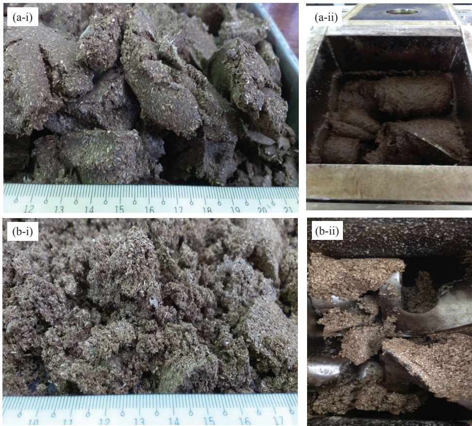
FIGURE 4. The mixture condition in the compounder at (a-i & a-ii) 40 wt. % and failure mixture at (b-i & b-ii) 50 wt. %
