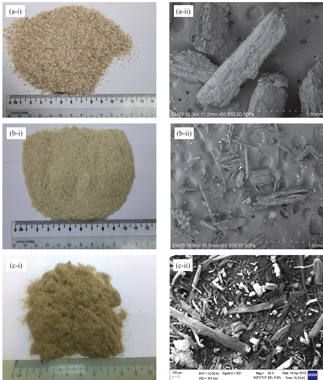
FIGURE 1. Image and SEM micrograph of kenaf filler: (a-i & a-ii) 20 mesh core, (b-i & b-ii) 40 mesh core, and (c-i & c-ii) bast
