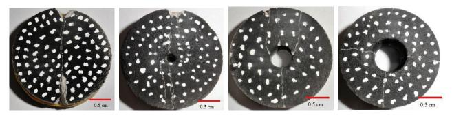
FIGURE 2. Mode of failure in a) solid, b) 0.1, c) 0.2 and d) 0.3 diameter ratio in ring disk under Brazilian test
