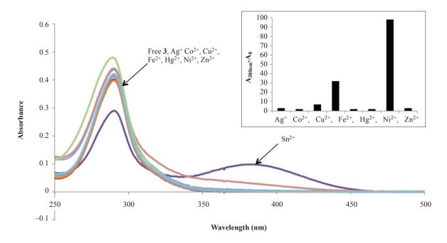
FIGURE 5. The absorption spectra of **3** upon addition of metal salts of Ag(OAc), CoCl<sub>2</sub>, Cu(OAc)<sub>2</sub>, FeSO<sub>4</sub>, HgI<sub>2</sub>, Ni(OAc)<sub>2</sub>, SnCl<sub>2</sub> and Zn(OAc)<sub>2</sub> (2 equiv) in 95% EtOH solution. Inset: Absorbance intensity at 380 nm, A<sub>380nm</sub> over that of blank solution of **3**, A<sub>0</sub>
