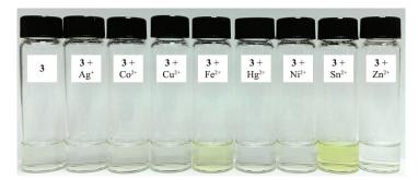
FIGURE 4. Colorimetric detection of **3** with metal salts of Ag(OAc), CoCl<sub>2</sub>, Cu(OAc)<sub>2</sub>, FeSO<sub>4</sub>, HgI<sub>2</sub>, Ni(OAc)<sub>2</sub>, SnCl<sub>2</sub> and Zn(OAc)<sub>2</sub>
