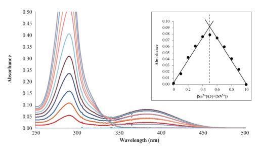
FIGURE 7. Job's plot of 3 and  $Sn^{2+}$  in 95% EtOH solution, with a total concentration of 20 mM ([3] + [ $Sn^{2+}$ ]) and a detection wavelength of 380 nm
