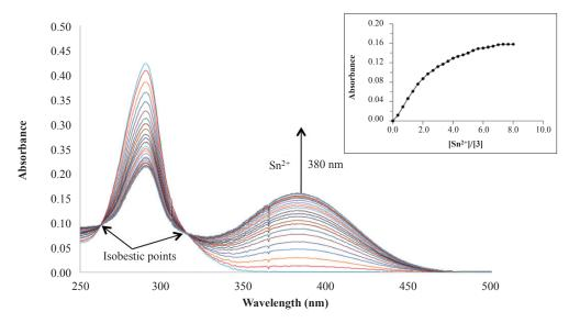
FIGURE 6. Change of absorption spectra of 3 (1  $\times$  10<sup>-5</sup> M) upon gradual addition of  $\text{Sn}^{2+}$  (1  $\times$  10<sup>-3</sup>M) ion concentration (10-250 mL) in 95% EtOH. Inset: Plot of UV-vis absorbance at 380 nm as a function of  $\text{Sn}^{2+}$  concentration
