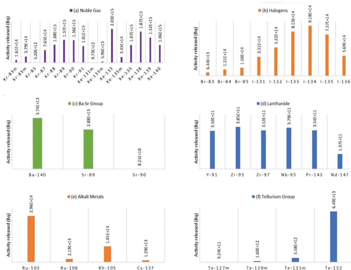
FIGURE 4. Source term (according to group) after a hypothetical severe accident at the partially damaged RTP
