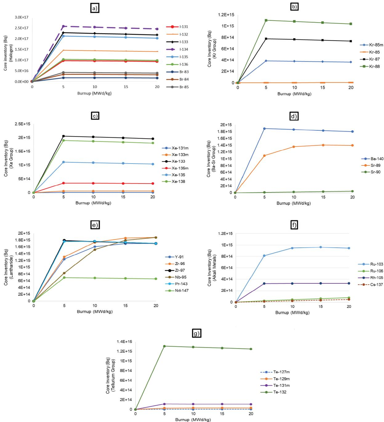
FIGURE 3. RTP core inventory in (Bq) for radionuclides in group (a) Halogen, (b) Noble gas: Kr group, (c) Noble gas: Xe group, (d) Ba-Sr group, (e) Lanthanide, (f) Alkali metals, and (g) Tellurium group versus burnup in megawatt day/kg (MWd/kg)
