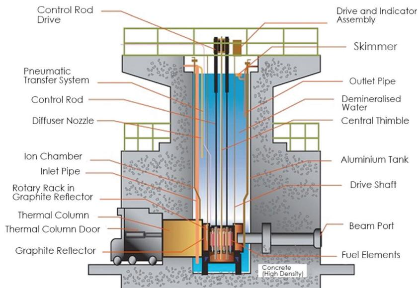
FIGURE 1. Cross section of the RTP facility
