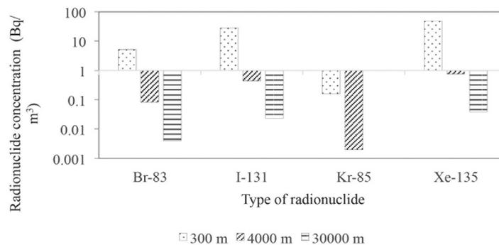
FIGURE 5. Radionuclide concentration based on distance on enrichment 20% for Category D (extreme raining or hot weather condition)
