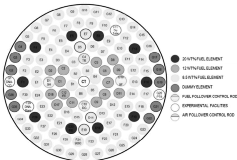
FIGURE 2. TRIGA MARK II Core-15 Configuration
