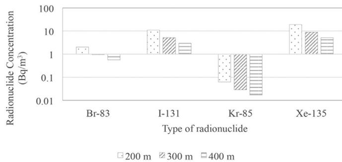
FIGURE 4. Radionuclide concentration based on distance on enrichment 20% for Category B (unstable yet neutral weather condition)
