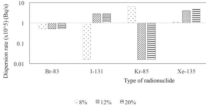
FIGURE 3. Chosen radionuclides dispersion rate on enrichment 8% for 86 fuel rods, 12% for 15 fuel rods and 20% for 10 fuel rods
