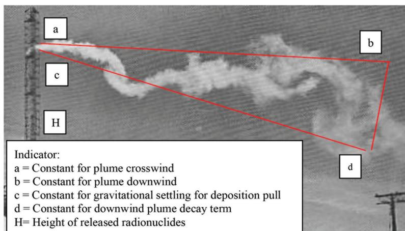
FIGURE 1. Plume shape consideration for atmospheric dispersion
