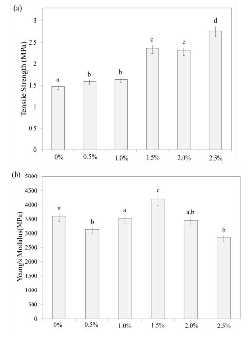
FIGURE 3. (a) Tensile strength and (b) Young's modulus of AM film with different concentration of thymol
