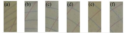
FIGURE 1. Appearance of AM active film incorporated with a) 0, b) 0.5, c) 1, d) 1.5, e) 2 and f) 2.5 % (w/v) of thymol
