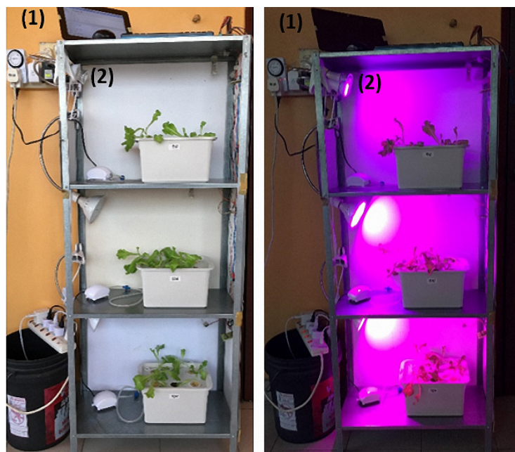
FIGURE 2. Set up of hydroponic system during day and night: (1) Raspberry Pi 2, and (2) supplemental red-blue LED light
