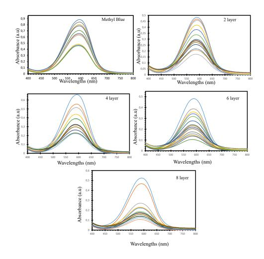
FIGURE 4. Absorbance spectra of methyl blue (a) without the Aldoped ZnO photocatalyst with various layers
