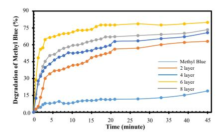
FIGURE 5. Photocatalytic activity of Al-doped ZnO thin film for the degradation of methyl blue
