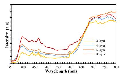
FIGURE 2. Photoluminescence spectra of Al doped ZnO thin film with various layer
