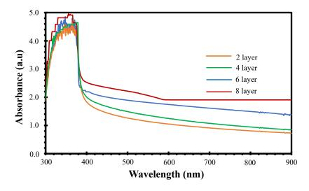
FIGURE 1. UV-Vis optical absorption spectra of Al-doped ZnO nanoparticle with various layer
