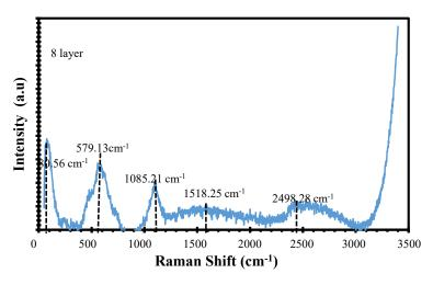
FIGURE 3. Raman spectra of Al-doped ZnO thin film deposited with 6 layers
