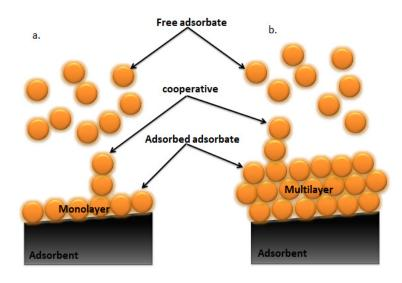
FIGURE 1. Illustration of adsorption process under monolayer (a) and multilayer (b)
