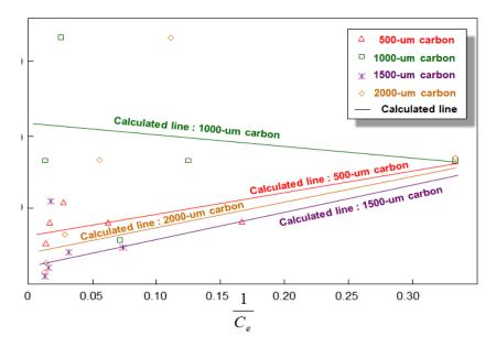
FIGURE 6. Langmuir adsorption isotherm model
