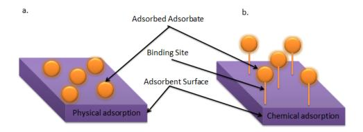
FIGURE 2. Illustration of interaction between adsorbate and adsorbent surface, (a) physical adsorption, and (b) the chemical adsorption
