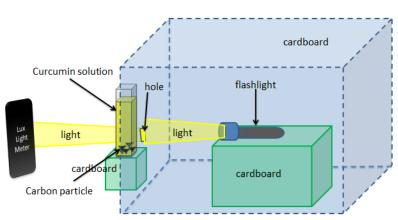
FIGURE 3. Carbon adsorption test by calculating the concentration of the solution
