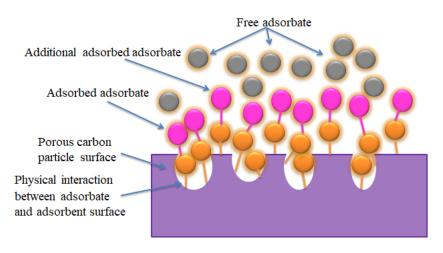
FIGURE 10. Illustration of adsorption process using carbon (as the adsorbent) and turmeric (as the adsorbate)
