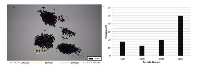
FIGURE 4. Microscope image (a) of carbon particles with their particle size distribution (b)
