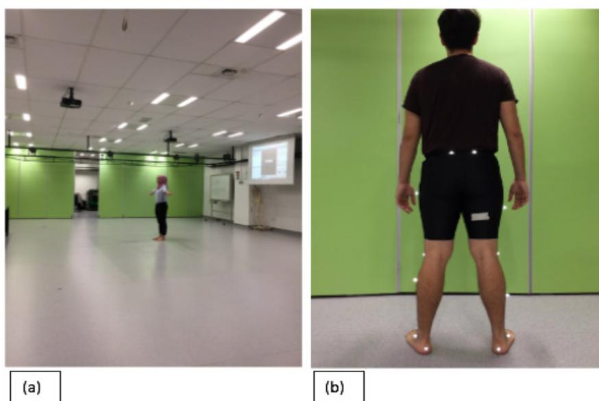
FIGURE 1. The experimental set-up; (a) The position of the subject during the T-pose procedure, and (b) The 16 passive markers positions on the lower limb of the subject
