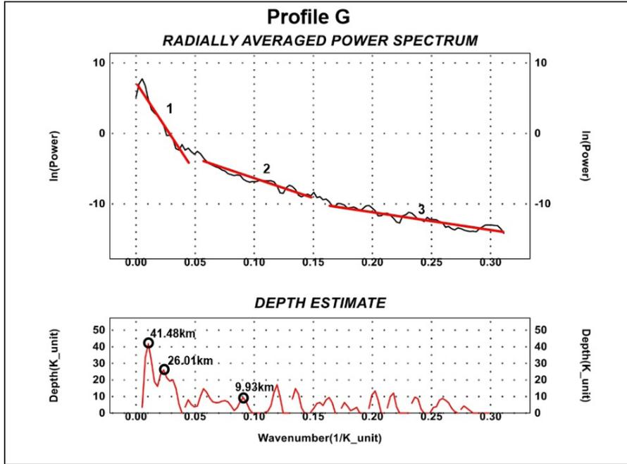
FIGURE 2. (g) shows the radially averaged power spectrum of profile G indicating the dominant slope of 1 to 3 and the depth curve indicating the depth of the slope
