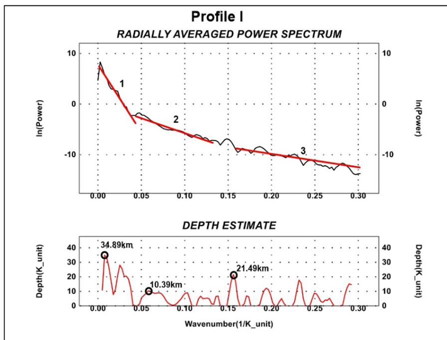
FIGURE 2. (i) shows the radially averaged power spectrum of profile I indicating the dominant slope of 1 to 3 and the depth curve indicating the depth of the slope
