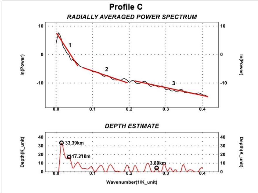
FIGURE 2. (c) shows the radially averaged power spectrum of profile C indicating the dominant slope of 1 to 3 and the depth curve indicating the depth of the slope
