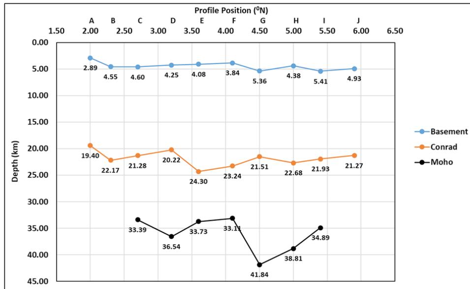
FIGURE 3. Depth variations of basement, Conrad, and Mohorovicic discontinuities based on spectral analysis of each profile from N-S of Peninsular Malaysia
