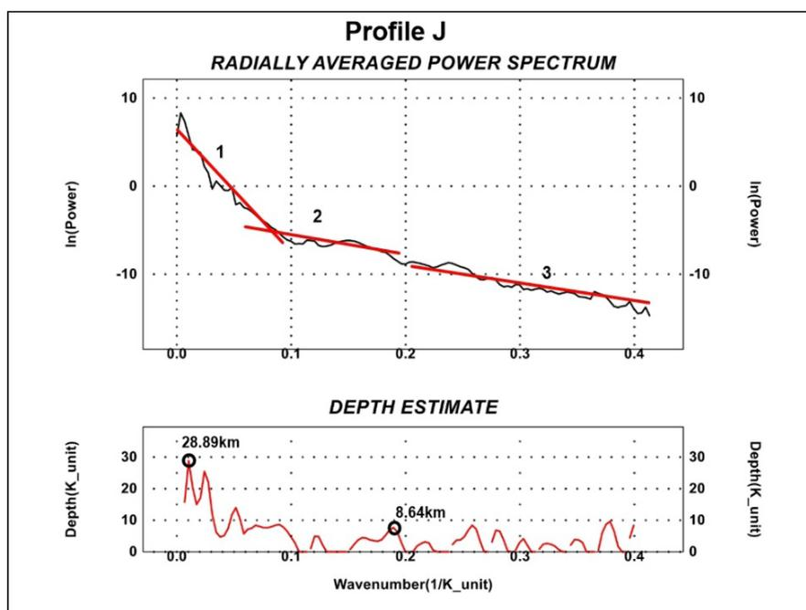
FIGURE 2. (j) shows the radially averaged power spectrum of profile J indicating the dominant slope of 1 to 3 and the depth curve indicating the depth of the slope
