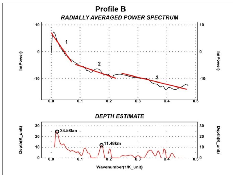
FIGURE 2. (b) shows the radially averaged power spectrum of profile B indicating the dominant slope of 1 to 3 and the depth curve indicating the depth of the slope
