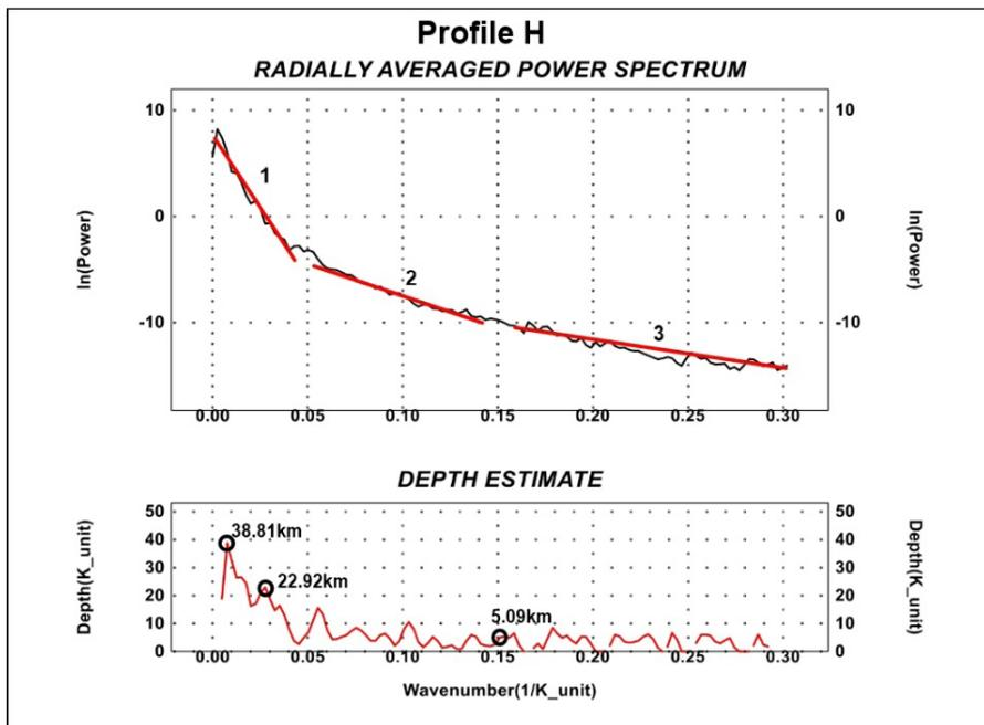
FIGURE 2. (h) shows the radially averaged power spectrum of profile H indicating the dominant slope of 1 to 3 and the depth curve indicating the depth of the slope
