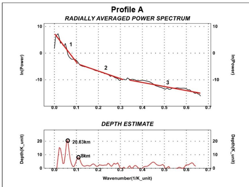
FIGURE 2. (a) shows the radially averaged power spectrum of profile A indicating the dominant slope of 1 to 3 and the depth curve indicating the depth of the slope
