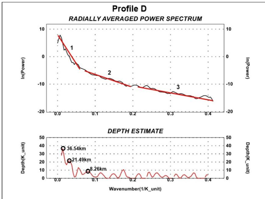
FIGURE 2. (d) shows the radially averaged power spectrum of profile D indicating the dominant slope of 1 to 3 and the depth curve indicating the depth of the slope
