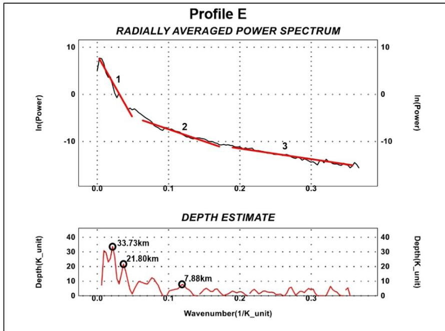
FIGURE 2. (e) shows the radially averaged power spectrum of profile E indicating the dominant slope of 1 to 3 and the depth curve indicating the depth of the slope
