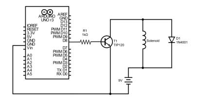
FIGURE 2. Circuit diagram of startle apparatus. The solenoid is driven by an Arduino Uno microcontroller to produce tap stimuli at the preset intervals
