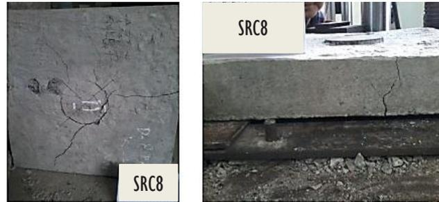
FIGURE 6. Crack pattern in SRC8 slab
