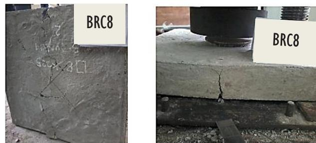
FIGURE 7. Crack pattern in BRC8 slab
