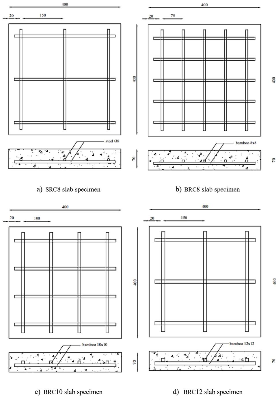
FIGURE 2. The details of slab specimens
