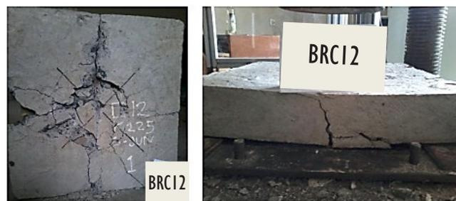
FIGURE 9. Crack pattern in BRC12 slab
