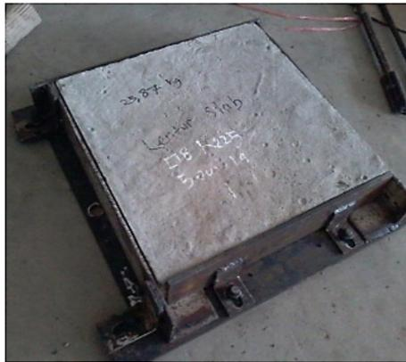
FIGURE 3. Slab specimen with fixed at four edges
