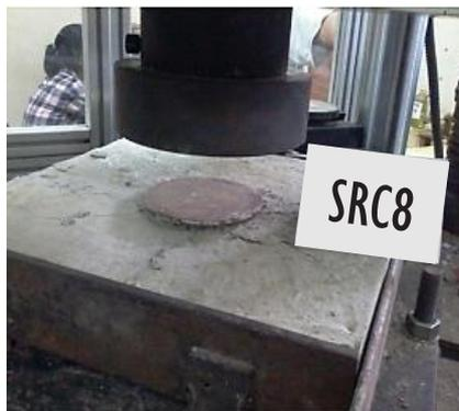
b) Concentrated loading configuration test
