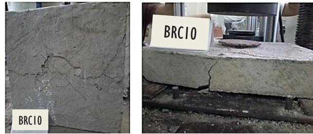
FIGURE 8. Crack pattern in BRC10 slab
