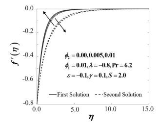
FIGURE 4.  $f'(\eta)$  along the shrinking cylinder  $(\lambda = -0.8)$
