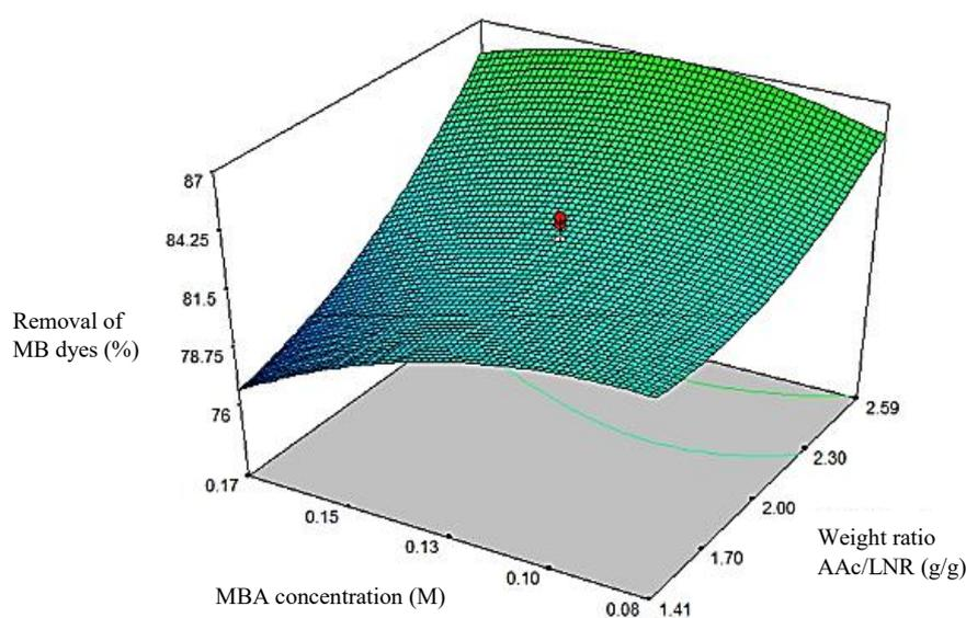
FIGURE 4. Response surface interaction between parameters weight ratio AAC/LNR and MBA concentration
