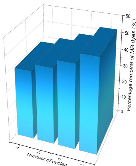
FIGURE 6. The reusability of LNR/AAC hydrogel for MB adsorption
