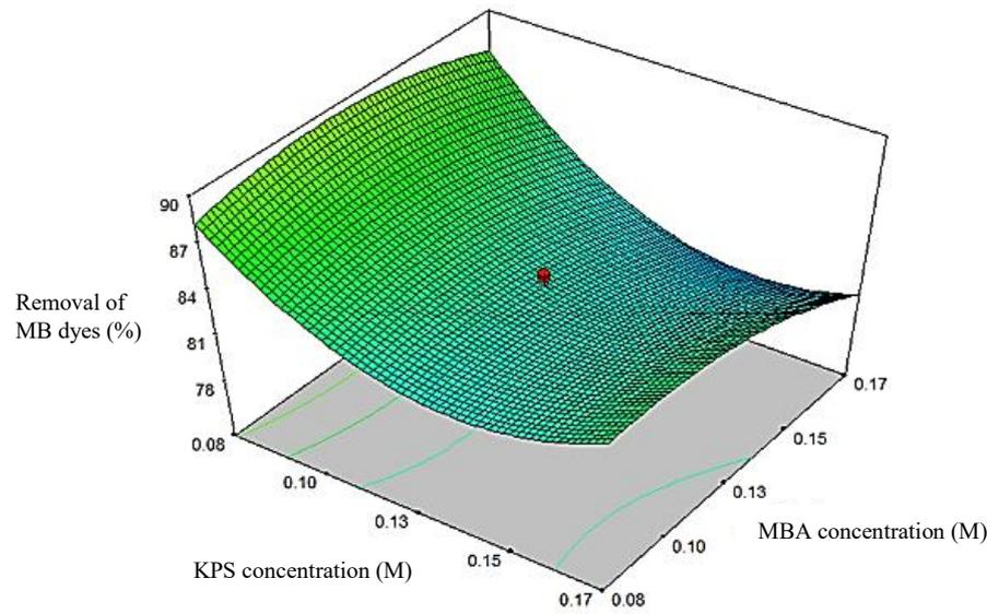
FIGURE 5. Response surface interaction between parameters KPS concentration and MBA concentration
