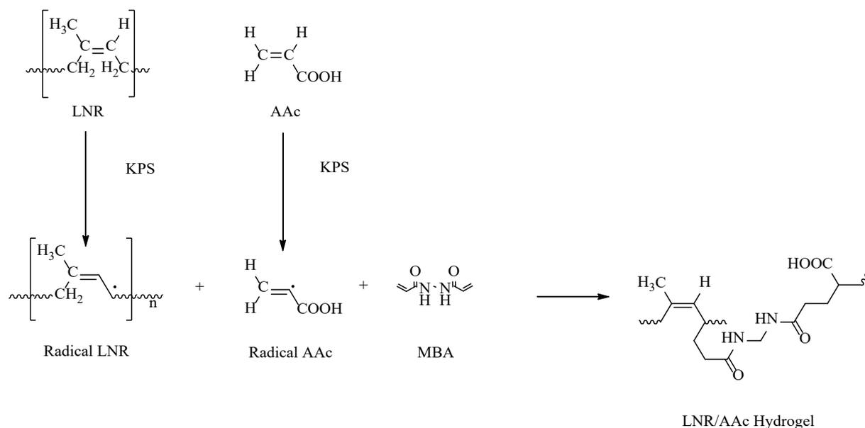
Scheme 1. Reaction scheme of LNR/AAC hydrogel (Firdaus et al. 2019)
