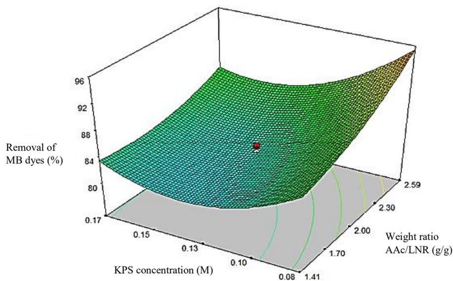
FIGURE 3. Response surface interaction between parameters weight ratio AAc/LNR and KPS concentration
