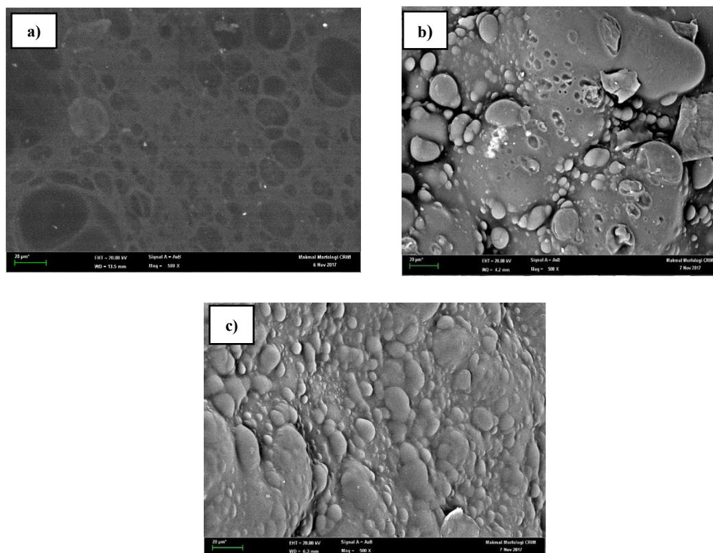
FIGURE 1. SEM images for surface of LNR/AAC hydrogel at concentration of MBA a) 0.01 M b) 0.06 M and c) 0.10 M at magnification of 500x
