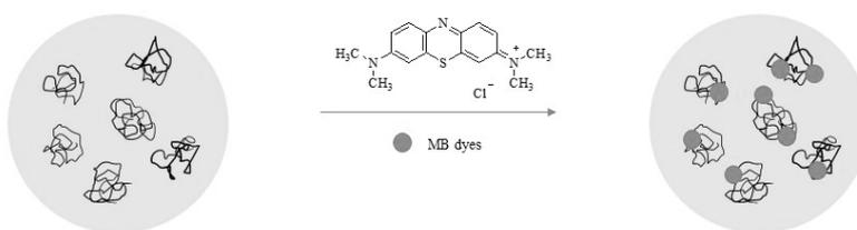
Scheme 2. Interaction mechanism between MB dyes and LNR/AAC hydrogel
