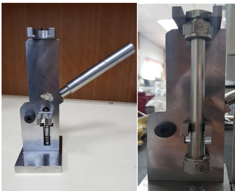
FIGURE 4. The actual custom-made reactor opener (left) and the reactor opener with reactor placed in it (right)
