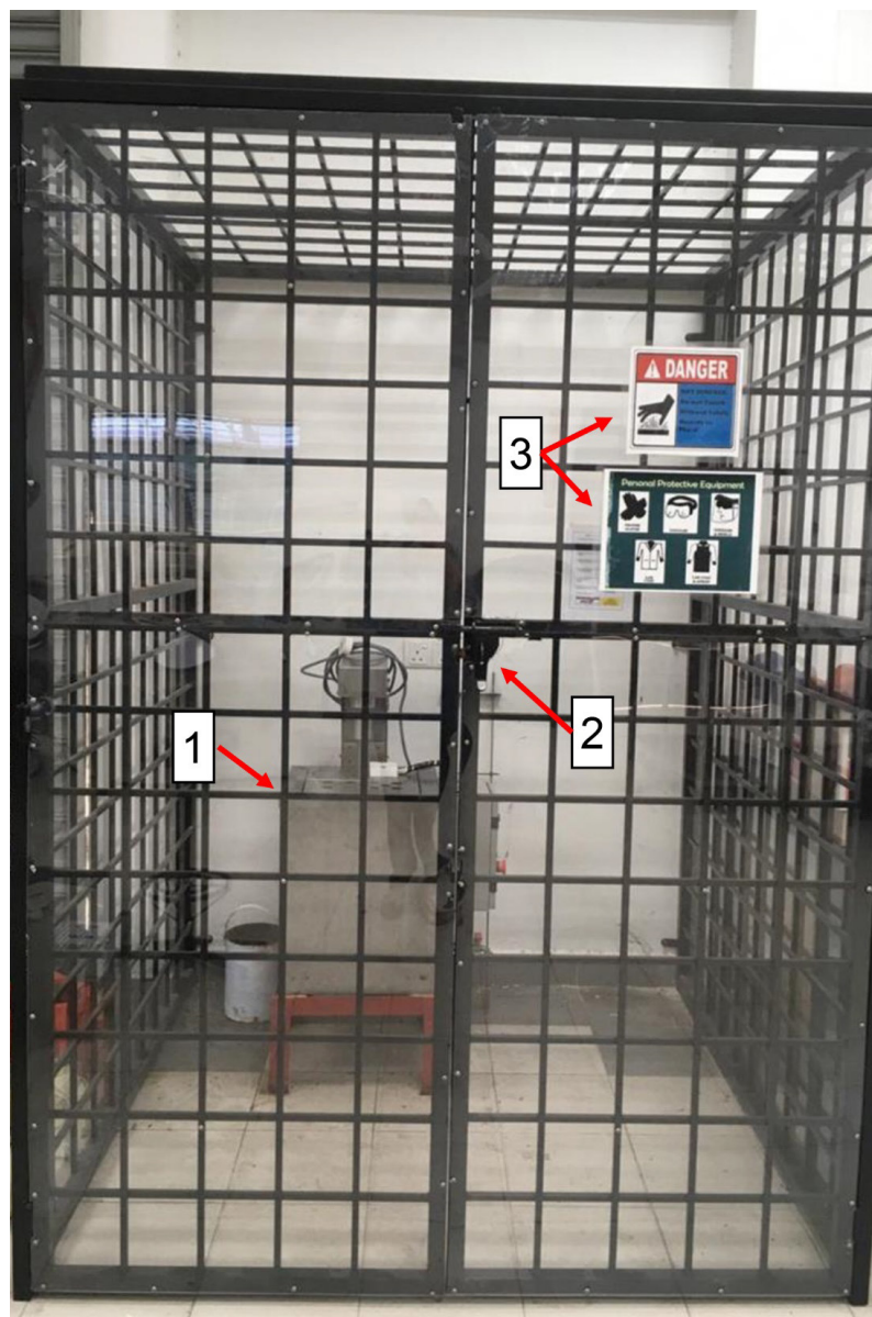
FIGURE 7. The safety cage for SWH with its components (1. Salt/oil bath; 2. Lock; 3. Standard operating procedures)
