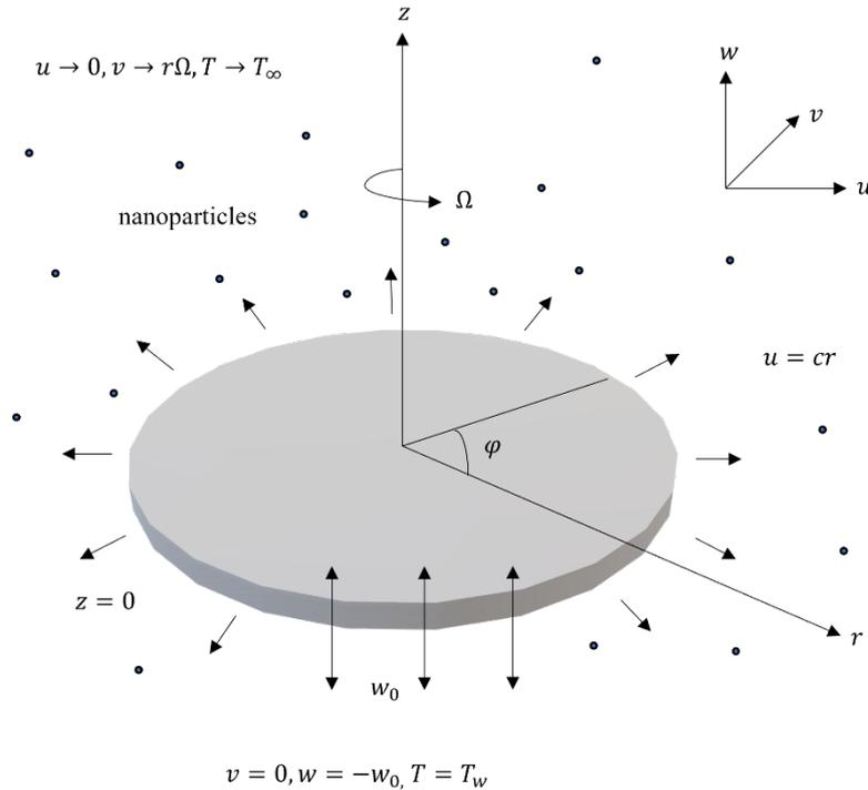
FIGURE 1. Physical model and coordinates system
