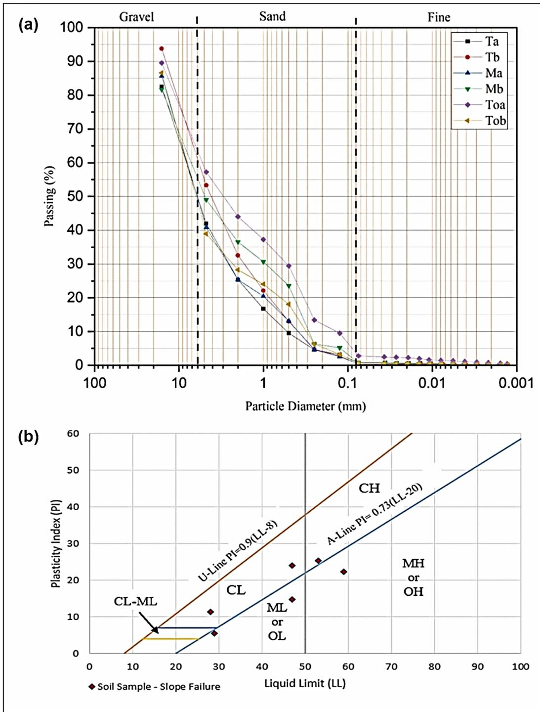
FIGURE 2. The figure illustrated (a) Particle size distribution curve; (b) Plasticity chart to determine the PI value of the soil samples
