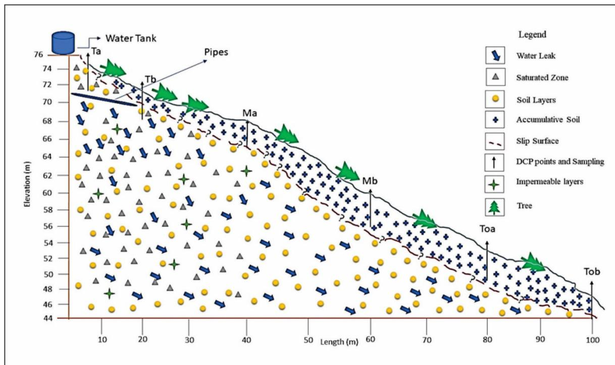
FIGURE 4. Cross-sectional view of the shallow landslide in UKM
