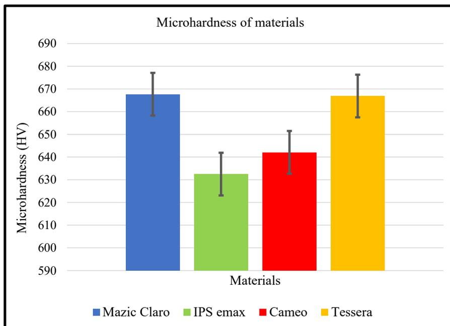
FIGURE 2. Microhardness of tested materials
