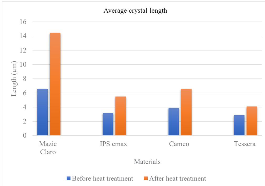
FIGURE 3. Average crystal length before and after heat treatment
