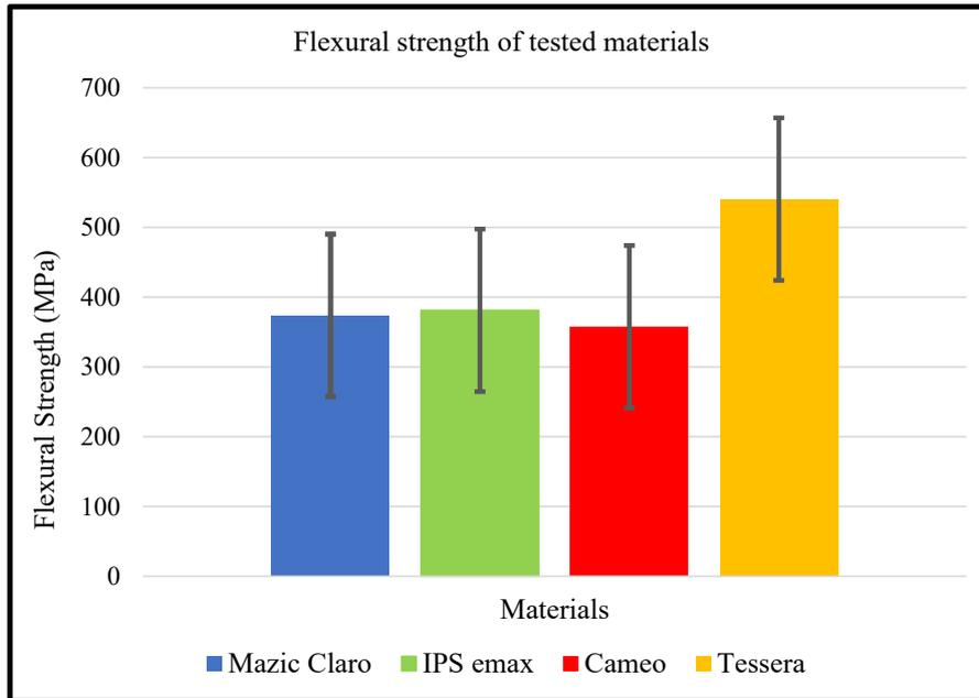
FIGURE 1. Flexural strength of tested materials
