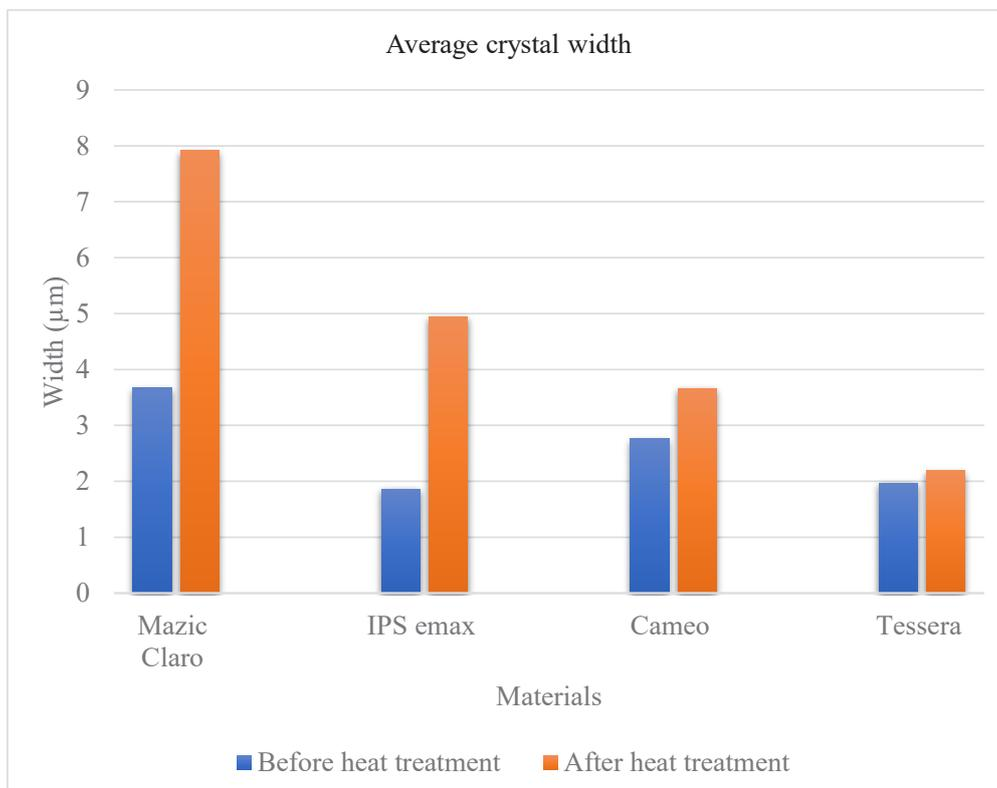
FIGURE 4. Average crystal width before and after heat treatment
