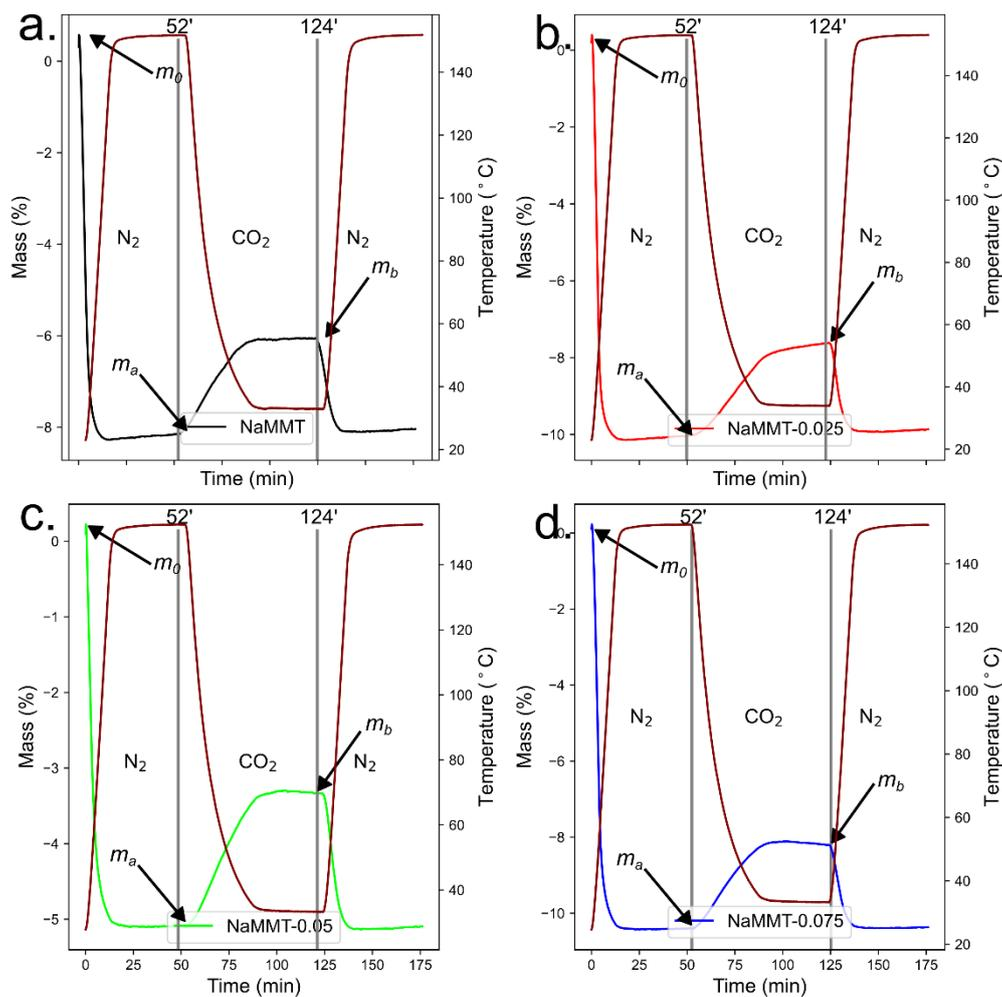
FIGURE 1. Mass and temperature change plot with respect to time for (a.) NaMMT, (b.) NaMMT-0.025, (c.) NaMMT-0.05, and (d.) NaMMT-0.075. The grey lines indicate the 52<sup>nd</sup> and 124<sup>th</sup> min position
