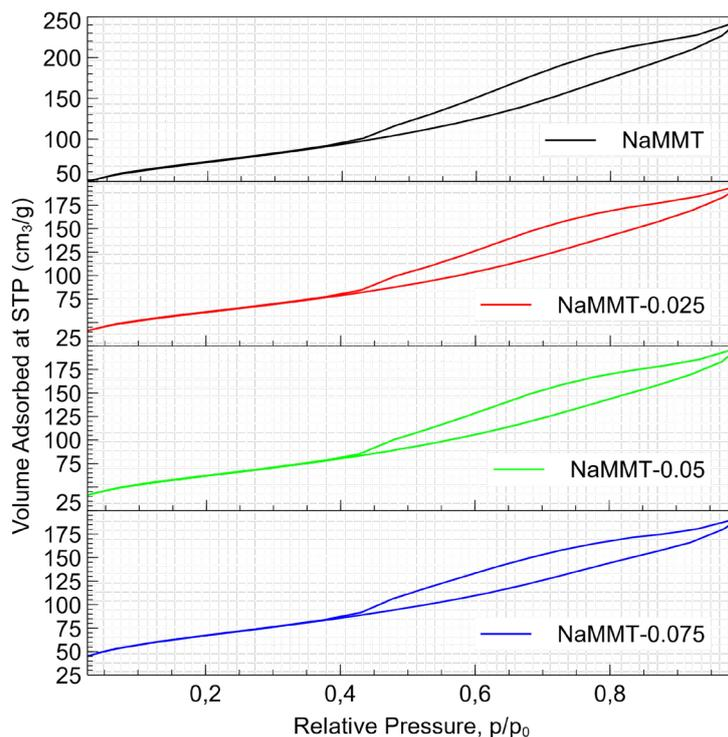
FIGURE 4. N<sub>2</sub> adsorption-desorption for all samplesTABLE 5. Pore parameters and CO<sub>2</sub> adsorption capacity of the samples
