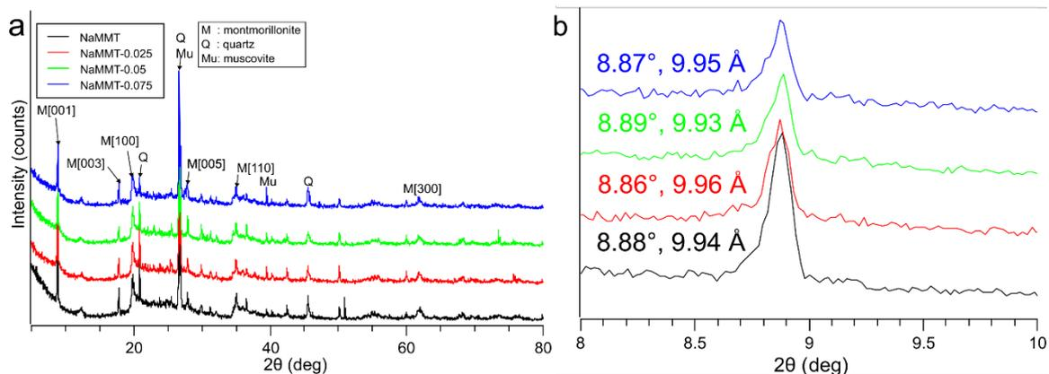
FIGURE 2. (a) XRD pattern for all samples. (b) The [001] peak and  $d_{001}$ , located at  $2\theta = 8.88^\circ$
