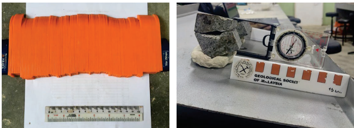
FIGURE 5. a) Example of Barton Comb with boulder's surface roughness profile and b) Example of tilt test
