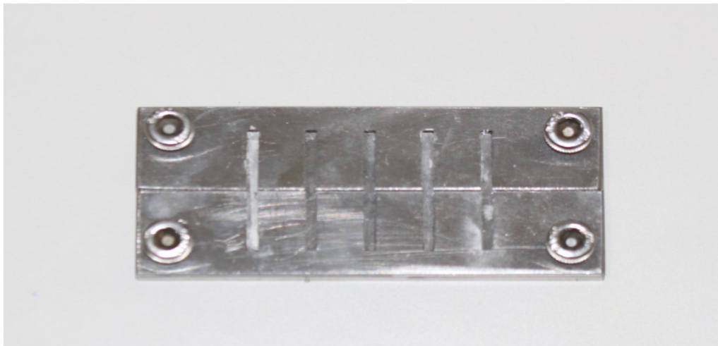
FIGURE 6. Customized stainless-steel mould for specimens preparation for flexural strength testing
