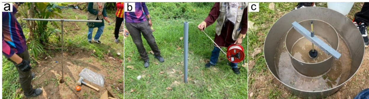
FIGURE 2. a) Soil sampling using hand auger, b) water table measurement, and c) double-ring infiltrometer test
